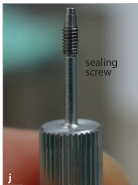
Fig 1j and 1k The sealing screw totally obstructs the channel due to friction and titanium features.
